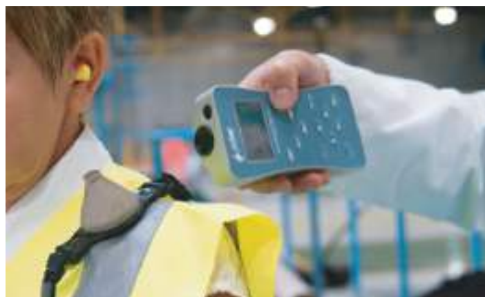
Noise dosimeters measure both the overall LAeq & LCPeak values as well as calculating daily personal noise exposure values in terms of LAep,d or LEX,8h
