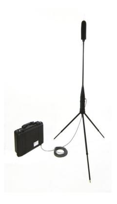
\*The WK2 has a hook system at the top of the tripod legs to allow this to be chained down. The hook is on a standard 20mm conduit thread so that all the standard electrical fittings can be utilised to fasten the system in place. Some users mount the microphone on a vertical threaded conduit tube to place it at a special height\*
