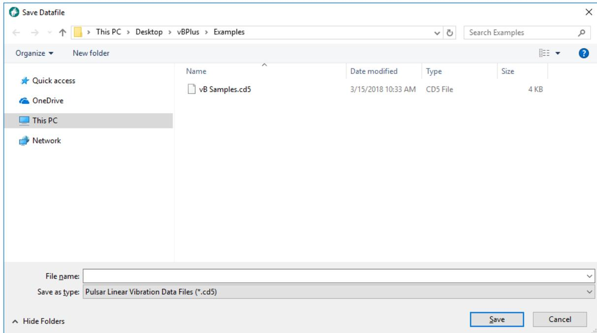
The initial default location for file storage is found under **Working Directories** from the **General tab** of **Settings**, this location can be changed if required, however vBPlus remembers the last folder location used enabling fast folder access.
