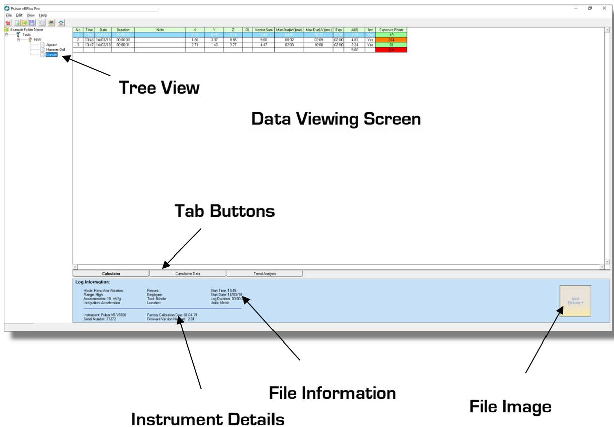
You will have the following selectable tab buttons at the bottom of the viewing screen: -
