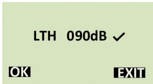
Set the desired level and enabled the alarm by using the arrow buttons. A tick denotes that the alarm is active; a cross denotes that the alarm is disabled. When set, press
