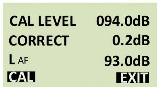
Use the arrow keys to set the CAL LEVEL to the acoustic calibration level (94.0dB for the MODEL106 calibrator).
